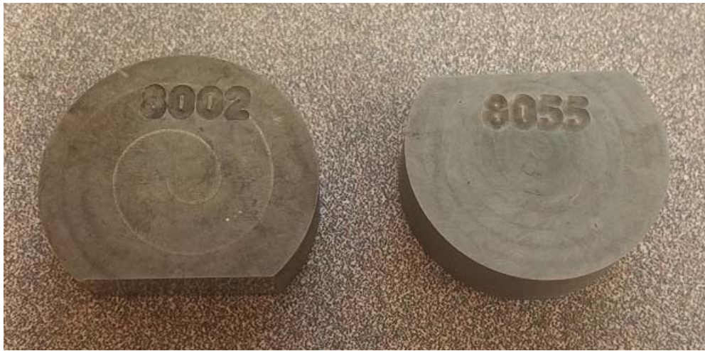
Figure 4.13 Hardened steel specimen 8002 and 8055
