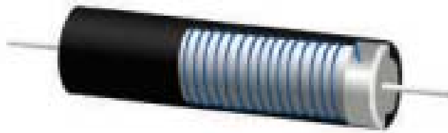
Figure 3.19 Construction of wirewound resistors. [41]
